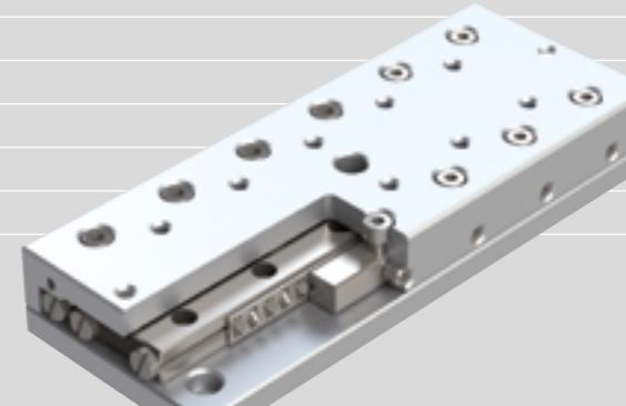
This steel crossed roller slide ([RT](#)) is also available in lightweight aluminium ([RTA](#)). Available with stroke ranges of 10–950 mm and a maximum load rating of 71.550 N.
