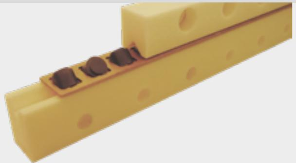
Fully ceramic linear bearing ([CR](#)) for applications requiring absence of magnetism, absence of lubrication or low mass combined with high stiffness. Commonly used materials are  $\text{Si}_3\text{N}_4$ ,  $\text{ZrO}_2$  or  $\text{Al}_2\text{O}_3$ . Typical fields of use include electron microscopy, semiconductor industry and medical applications.
