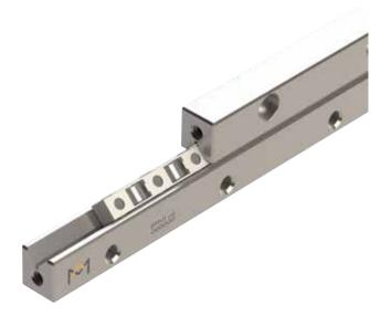
Linear bearings type RSDE are a next generation development of the RSD type. The deeper V-groove in combination with the high density roller cages offer higher load ratings and stiffness without changing the boundary dimensions of the rails. RSDE linear bearings are used mostly in highly dynamic applications requiring high speed, high running accuracy and outstanding quality.
